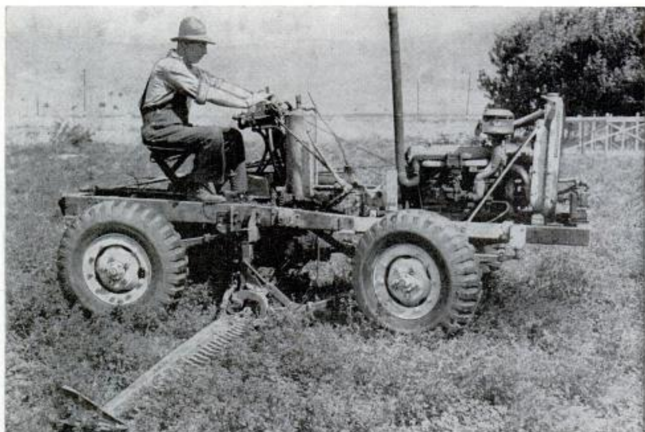
Operator of ranch-designed mowing machine controls all four wheels, brake, clutch and cutter bar by hydraulics
